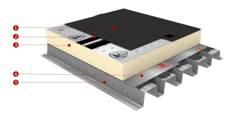
Firestone's EPDM RMA System is a lightweight, non-penetrating mechanically attached system developed around the QuickSeam™ RMA strip: a strip of reinforced EPDM membrane incorporating two strips of self-adhesive QuickSeam Splice Tape laminated along each edge over the length of the strip.
