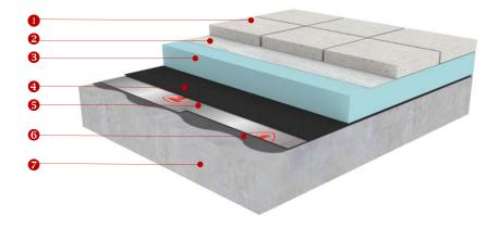
Firestone's Inverted System is a variation of the conventional ballasted system. It is ideal for roofs with regular traffic, or roofs in severe weather climates. It can be applied on any building that can accommodate the extra load of the ballast and where the roof slope does not exceed 10%.
